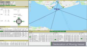
ESM data captured by the MicroESM sensors is streamed back to ESROE's multi-sensor hub, hosted on a remote computer, allowing triangulation of bearing lines to provide an accurate indication of range.
