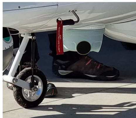
Redesigned with a very low SWAP, MicroESM can be UAV-mounted (see feet for size comparison)
